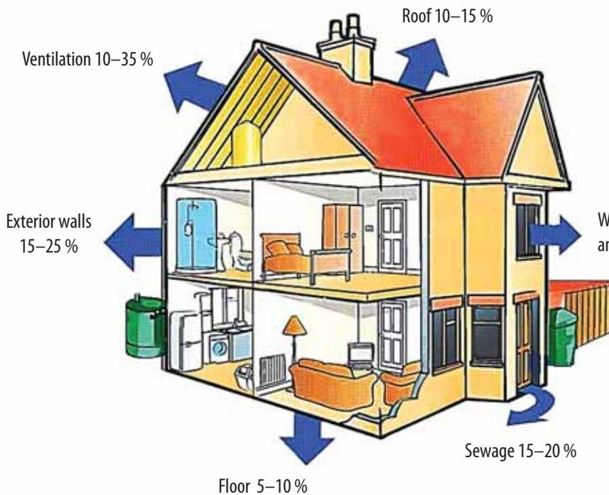
Energy losses in buildings can account for up to 70%. These losses can be reduced by owners or management companies. Basically these are losses of heat.
